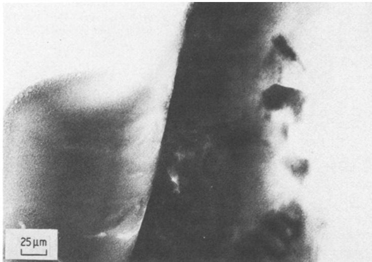
Figure 3 TEM bright-field image of the interface region between fibre and matrix in a composite containing 10 wt % Mg.
